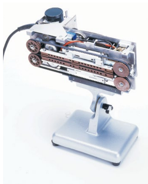
Inside mechanics of the HS-BII Hand Sealer
